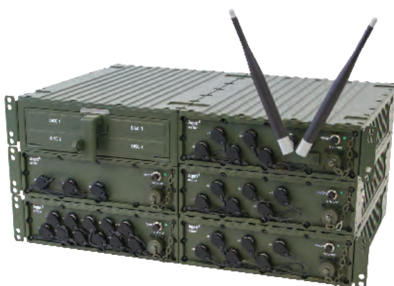
Aqeri mini-series stacked for rack mounting together in pairs
