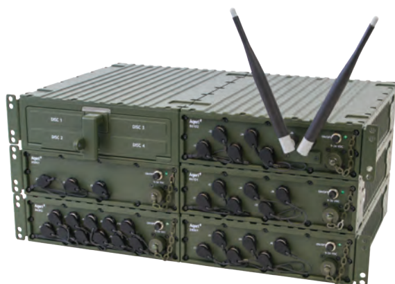
Aqeri mini-series stacked for rack mounting together in pairs
